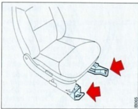
Mounting lugs for child seat that requires an under-mounting strap (cars without passenger-side airbag)
