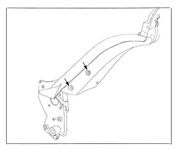
c. Side rail lying on main motor - balance link bent?
