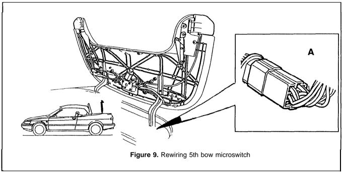
NOTE: Some cars have had the wiring modified per instructions included herein but have not had the microswitch removed. If upon inspection you can determine that the wiring is correct, remove the microswitch and tape and secure the connector.
