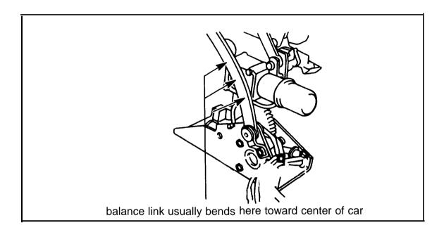
If the balance link is bent, also inspect the control arm on both sides for bending.
