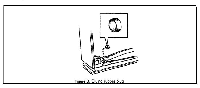
Glue the rubber plug, P/N 46 96 175, to the head of the pop rivet securing the second bow's stop. See Figure 3.C.
