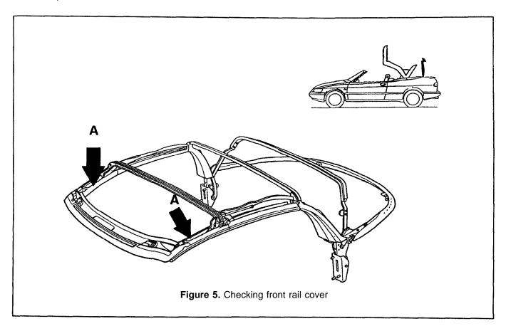
1. Remove any loose front rail covers and touch up with flat black paint as needed. The Factory has determined that these covers are not necessary.
