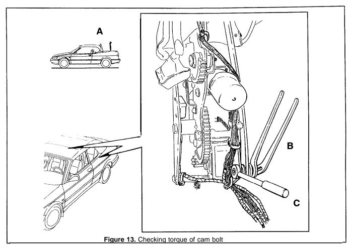
Tighten cam bolts to 23Nm.
